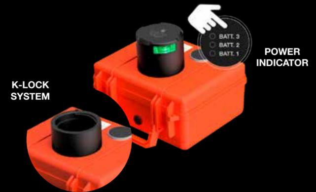
The K-lock system enables you to change the navigation light function in seconds. Any standard (circular) Lopolight navigation light can be fitted. The daylight switch function is calibrated to switch the navigation light on/off at 100/200Lux – as specified by rules and regulations. Typical battery lifetime is 25 days.
